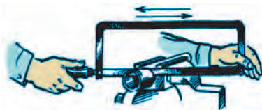
60-rasm. Trubalarni chilangarlik arrasi bilan qirqish.
